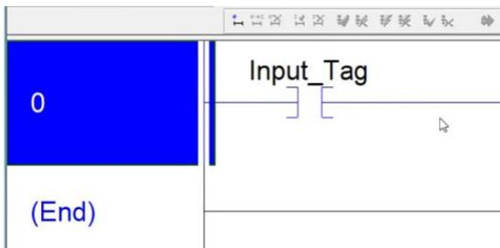
Now the ladder code rungs display as continuous lines with no warnings. This indicates the code is ready to execute.
