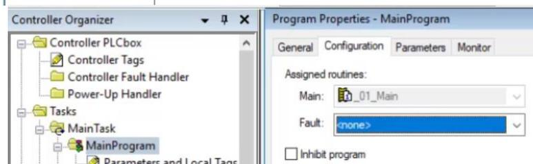
Here we are looking at the properties of the code module MainProgram. The code module `_01_Main` is listed as the main assigned routine of the MainProgram module.
